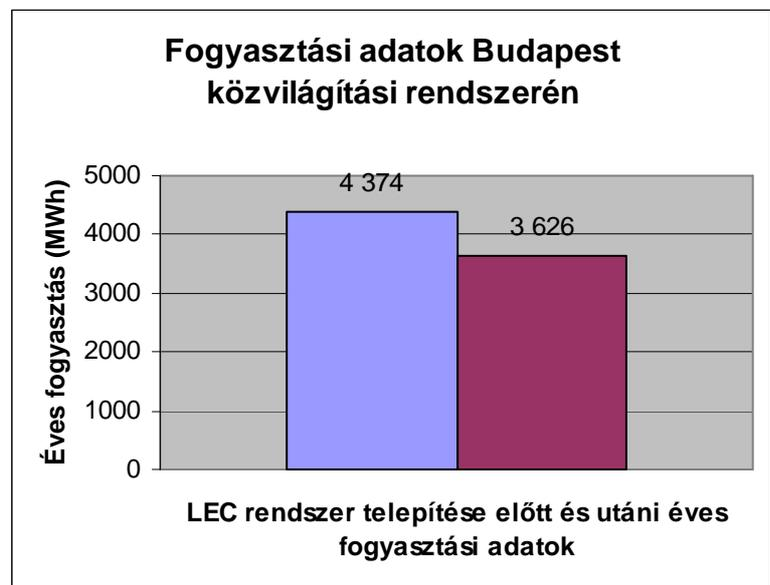
Currently there are measurements in process of certain transformation circles, where LEC devices could be installed in the near future in order to save energy on the Budapest public lighting network.
